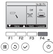
Press the  $\boxed{F4}$  button to turn the louver swing ON and OFF.
